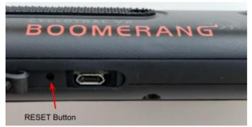
Using an unfolded paperclip, gently press the RESET button twice within 1 second (double-click the button).
