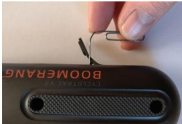
Confirm that the Cyclotrac is ready for USB upgrade by observing the green light near the gear icon. The green light should smoothly fade on/off. No other lights should be on.
