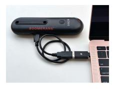
Cyclotrac will be detected as a USB disk with the name "BP600BOOT". Your operating system may automatically install drivers to support the USB disk. This may take up to ~2 minutes.
