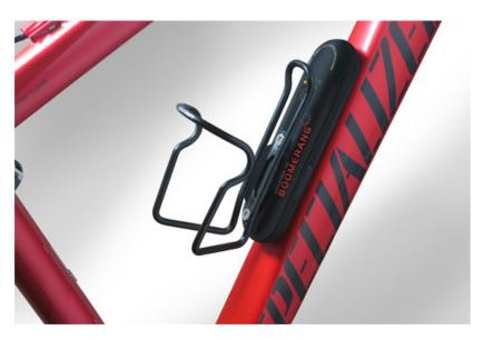
Use the supplied screwdriver bit to tighten the screws. Tighten the screws until the Cyclotrac and bottle cage are held securely to the frame and the screws cannot be loosened by hand. Take care not to overtighten screws, because that could damage the device or bike.
